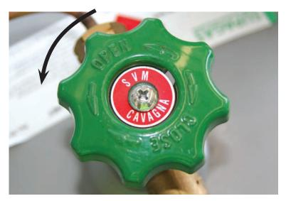
Ensure that the valve on the 45kg LPG cylinder is turned open in the direction of the arrows.
