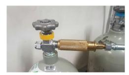
Typical Hose Connection on Cylinder in Use
